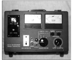
Fig. 33 Toshiba Portable Vacuum Checker
